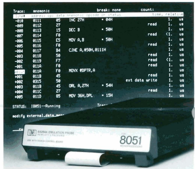
This new emulator for the Intel 8051 microprocessor directly monitors the microcomputer's internal bus and displays information about the emulator's activity.
